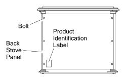
Figure 6 - Removing Back Panel
